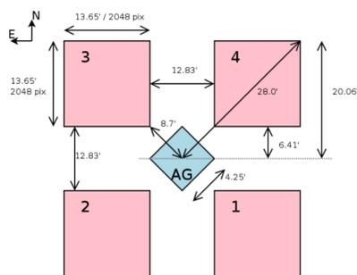
Figure 2. The WFCAM focal plane, showing the four Rockwell Hawaii-II 2048 x 2048 pixel detectors, spaced by 94%, with an optical guide camera centered between the arrays.
