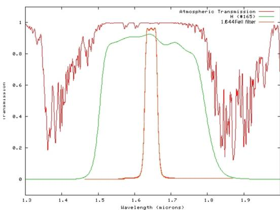
Figure 1. This image shows the filter profiles for the WFCAM broad band H filter and narrow band 1.644  $\mu\text{m}$  [FeII] filter along with an atmospheric transmission profile for reference.
